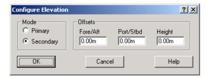
Assign the vehicle's height or depth by selecting the Primary or Secondary radio button on the dialog. In the Vehicle Text window, a vehicle's elevation (ELEV) will have the opposite sign of its depth (ROV D). The Height offset will be subtracted from the observed value. All the offsets are used for pitch and roll corrections.
